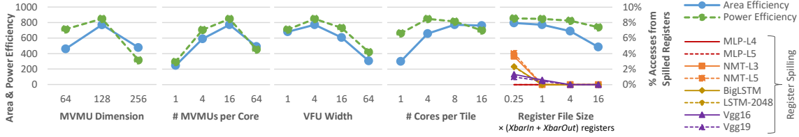
Figure 12. Design Space Exploration: Tile Area Efficiency in GOPS/s/mm 2 and Tile Power Efficiency in GOPS/s/W
